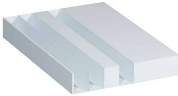
Figure 1.3: Example sound diffuser using quarter-wavelength resonators, or wells.
